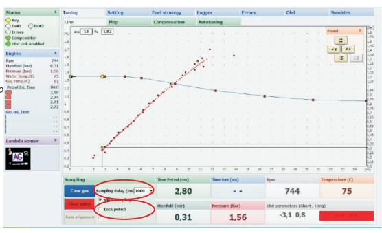
After creating a petrol map, switch system to gas and create a **gas map** in exactly the same way as petrol one.
