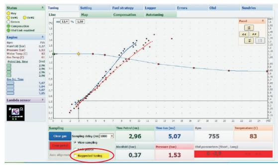
On the chart there will appear green points suggesting what the model should look like for the petrol and gas maps to overlap. At this point, the model must be adjusted. You can do this in two ways: using the automatic Auto alignment function or you can do it manually. Deciding for manual adjustment, by "pulling" individual regulatory model points you lead a line as close as possible to the green points, gently, with no sudden curves.
