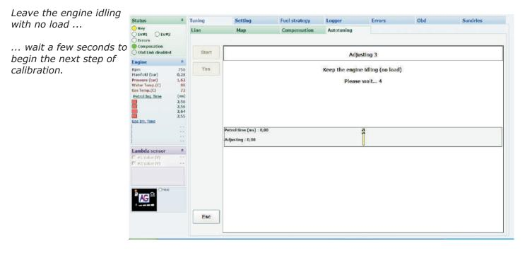
The system checks the petrol injector opening times and the stability of engine load. In the absence of apparent stability the message on the right appears. Please check what is causing the instability, remove it, then use the **Continue** button to check the stability again. If you use the Ignore button, the system will move to the next step without rechecking stability, which may affect the quality and accuracy of the calibration.
