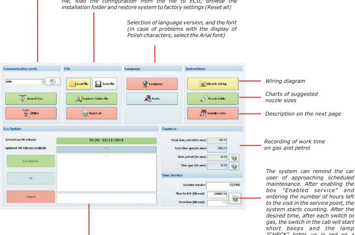
System Zenit Pro software lets you upgrade the firmware of the ECU. With Dual Memory function, this process is completely safe. For successful update you need to ensure stable power supply conditions. A special wizard guides you step by step through the update process.
