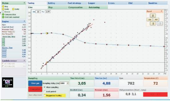
When there are discrepancies, the correction procedure should be performed. We do this by selecting the **Suggested tuning** (this option activates automatically and highlights in yellow when we collect a sufficient number of map points).
