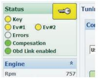
To make changes to the system settings, click on the button with a key symbol and then a window appears to enter a password and temporarily unlock the system (until you disconnect from the ECU)
