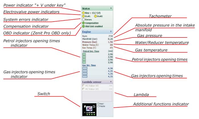
The information panel is located on the left side of the program window, it is available irrespective of the chosen tab and it enables watching the basic system parameters:
