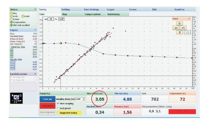
In the example above, the petrol injection time at low rpm is 3.05 ms. After changing to gas supply, the time should be within 3% error which should be from 2.95 to 3.13. If this difference is greater, it must be corrected by setting using the tab **Tuning -> Map**.
