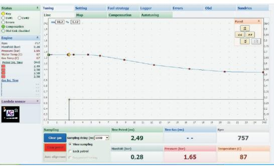
We start collecting the map when driving "on petrol". For the map points to be visible in the program you must select View sampling. **Regardless of whether** the function is active, the map points are collected and stored in memory. Points are "collected" with different loads but only when the temperature of the reducer is above the value set at Setting> Change-over Parameters> Water Temperature
